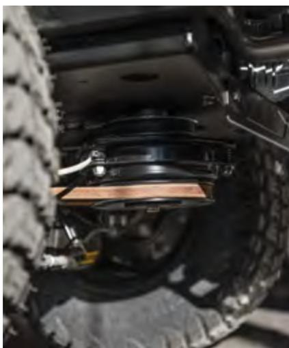
Soft start clutch to reduce stress on the mower's engine, belt, and components.
