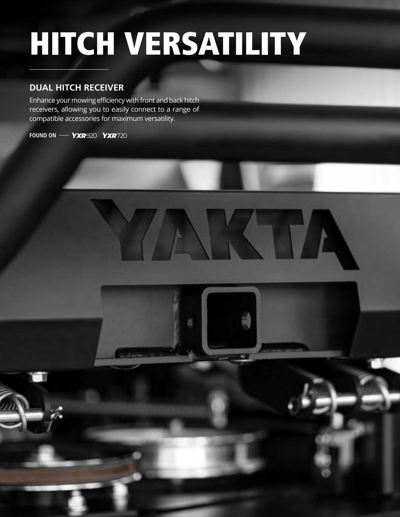
A close-up, black and white photograph of a YAKTA machine's dual hitch receiver. The word "YAKTA" is prominently displayed in large, bold, black letters on a dark metal plate. Below the name, a rectangular metal receiver is visible, designed for attaching accessories. The background shows the blurred mechanical components of the machine, including what appears to be a blade and various bolts and nuts.
