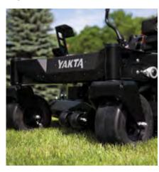
A reinforcement plate, bullnose front end, and bumper on the deck that adds protection.
